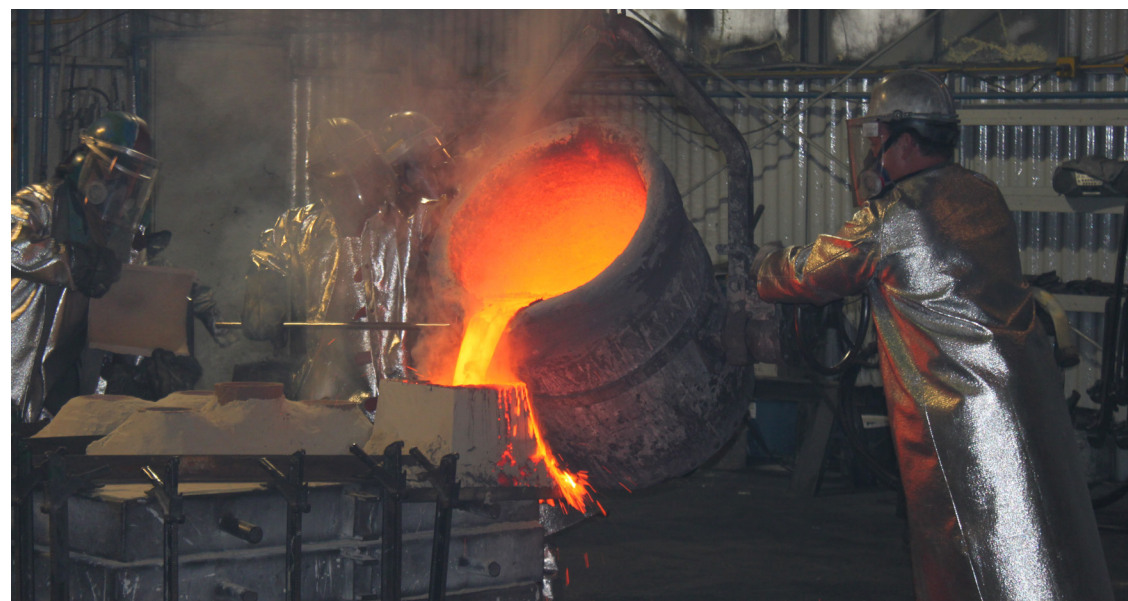
Calumet Brass Foundry workers pour 2,400 pounds of C93800 into a sand mold.
